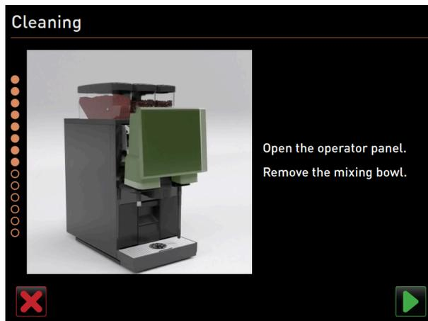
Figure: Lifting user panel
