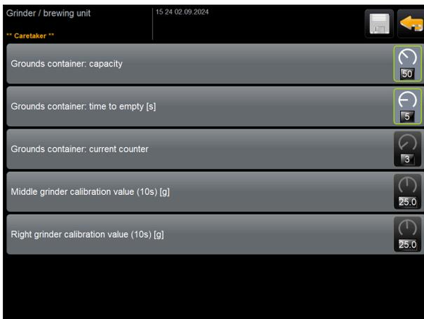
Figure: Screen with settings for grinder/brewing unit
