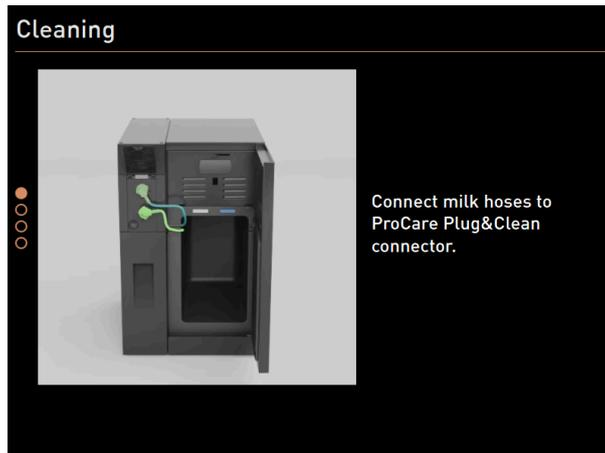
Figure: Connecting milk hoses to **Plug&Clean** connections
