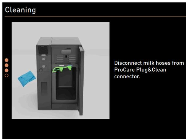
Figure: Removing milk hoses from **Plug&Clean** connections
