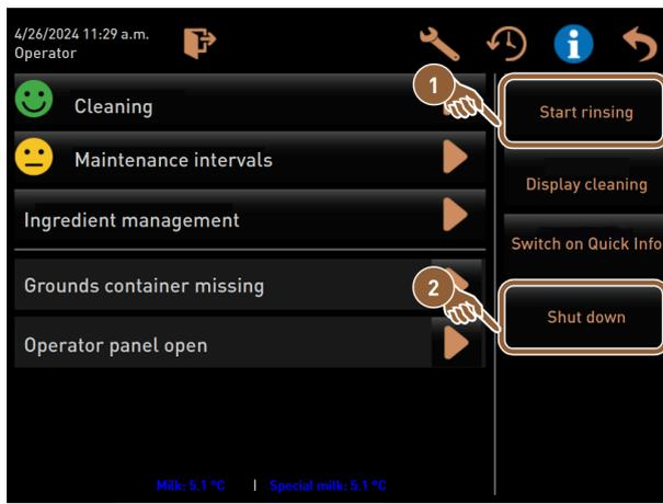
Figure: Switching off using touch screen
