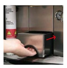
**8.** Put back metal shield and slide coffee grounds bin back into place.
