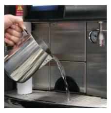
**12.** Flush drip tray with a pitcher of water. Wipe the machine exterior thoroughly with a clean, damp cloth to remove residue.
