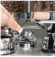
Lift dome lid and drop in one Schaerer cleaning tablet. Close lid after dropping tablet. Note: Dome lid is located behind front center hopper for 3 grinder machine confi guration.
