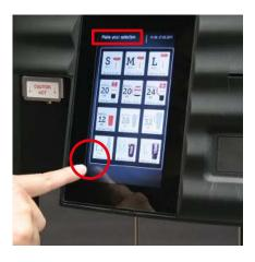
2. When the "Start cleaning" message appears on the upper left corner. Press and hold (3-5 seconds) the lower left corner of the touch screen to bring up service menu.
