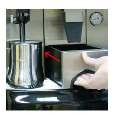
7. Put back metal shield and slide coffee grounds bin back into place.
