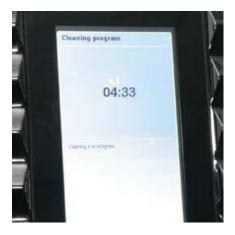
9. Press "Continue" on the screen to activate cleaning cycle. Cleaning runs (4:33 min.)
