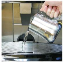
11. When automated cleaning cycle is complete, flush drip tray with a pitcher of water. Wipe the machine exterior thoroughly with a clean, damp cloth to remove residue.
